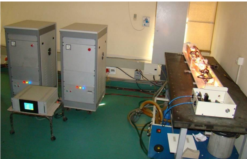
Specially Developed Nd:YAG Laser 500W(avg)
