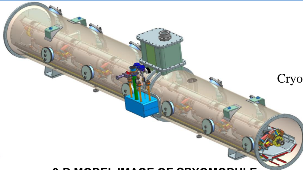
3-D MODEL IMAGE OF CRYOMODULE 2c (Showing major sub-systems in Cryomodule w/o piping)
